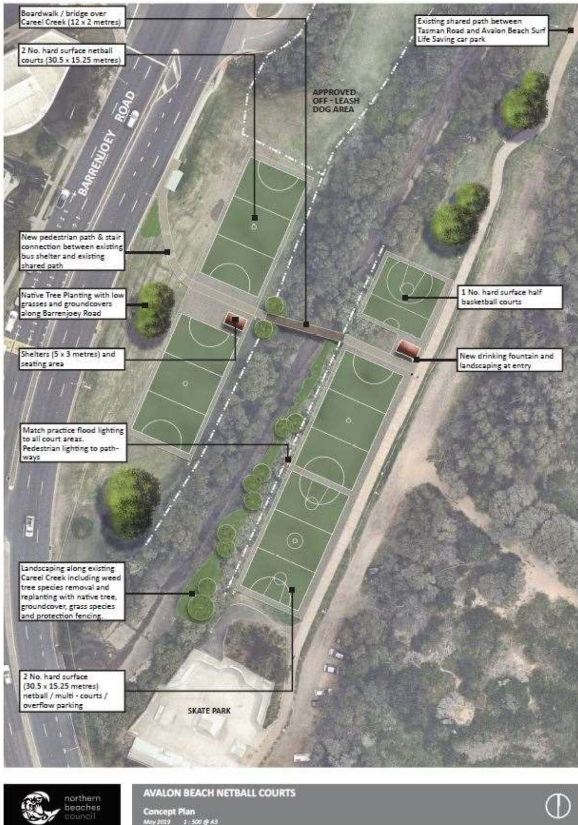
Figure 4 Concept plan for proposed sports courts at Avalon Beach Reserve in the Draft Plan of Management
